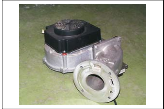
Fig.: Visual check, non-return valve.
