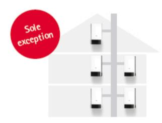
Non-condensing technology (type B1) can still be installed here. Single appliance: open flue, chimneyvented, non-condensing appliance with non-return flue gas damper, e.g. CGU-2K
