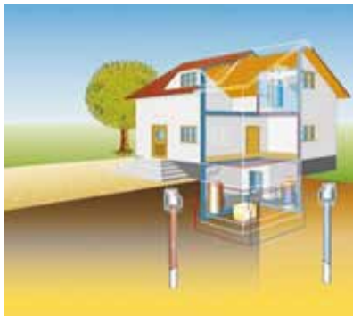
System scheme – extraction and absorbing well
